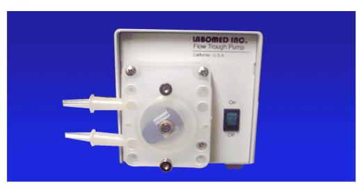
The Flow Through System Pump is fixed-speed, self priming peristaltic pump. The peristaltic pump roller pressure squeezes fluid through the tubing. The flow is proportional to the speed of the rollers (rpm) and the inside diameter of the tubing).
